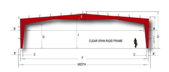
The clear span primary framing is similar in prefab buildings
